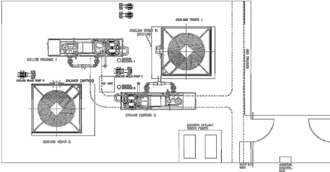
Figure 9. Plant Room Layout Showing NH<sub>3</sub> Chillers and Cooling Towers
