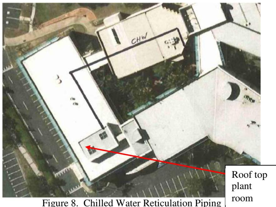
Figure 8. Chilled Water Reticulation Piping
