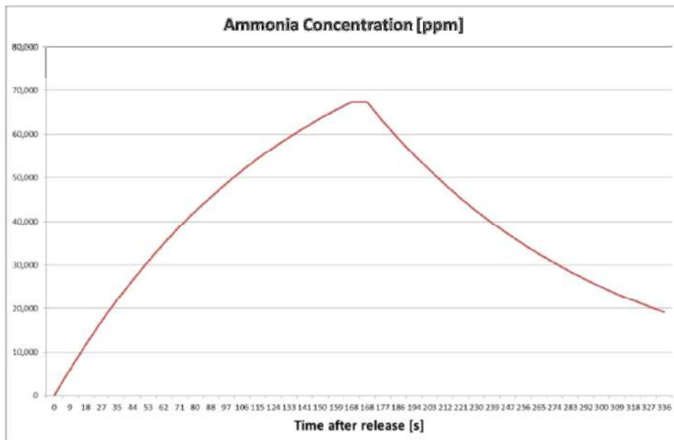
Figure 10. Ammonia concentration as a function of time in the event of a catastrophic release of an entire refrigerant charge (33 kg) in liquid form.
